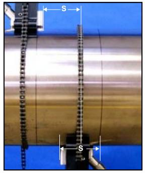
Figure 3-21: The Installed CFG-PI Fixture, with Calculated Spacing
